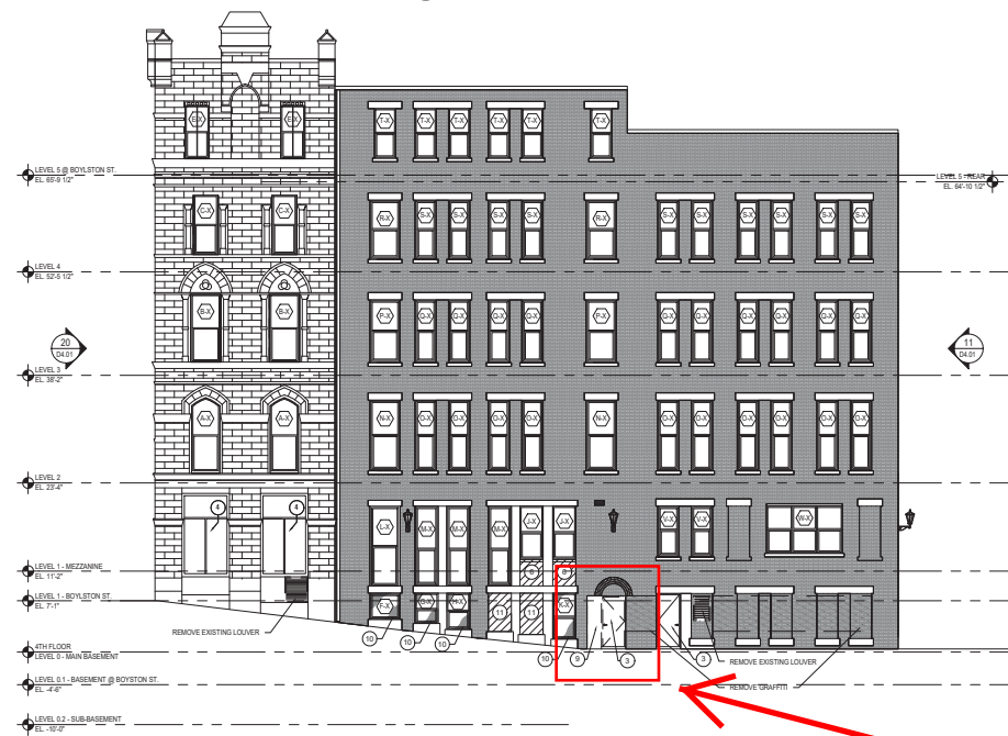
10 WEST ELEVATION - DEMOLITION Scale: 3/32" = 1'-0"
