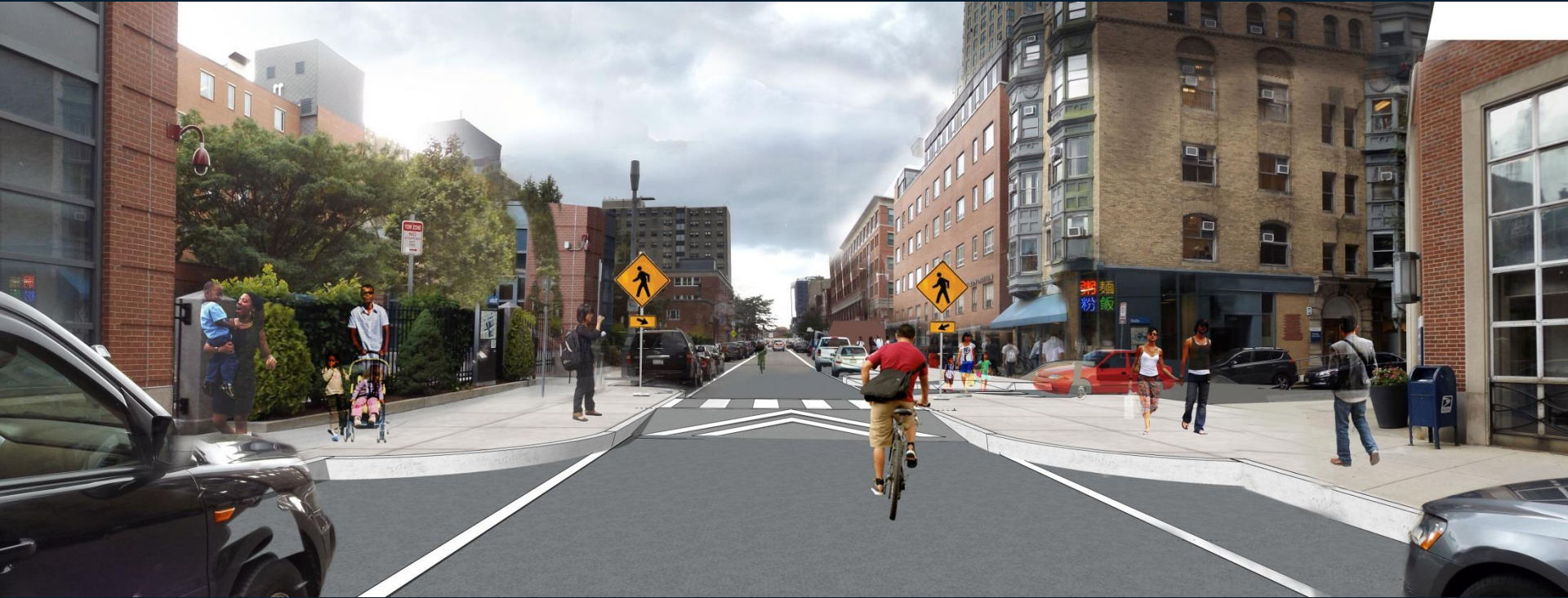
Rendering of a raised crosswalk at the example intersection, Harrison Ave and Bennet St.
