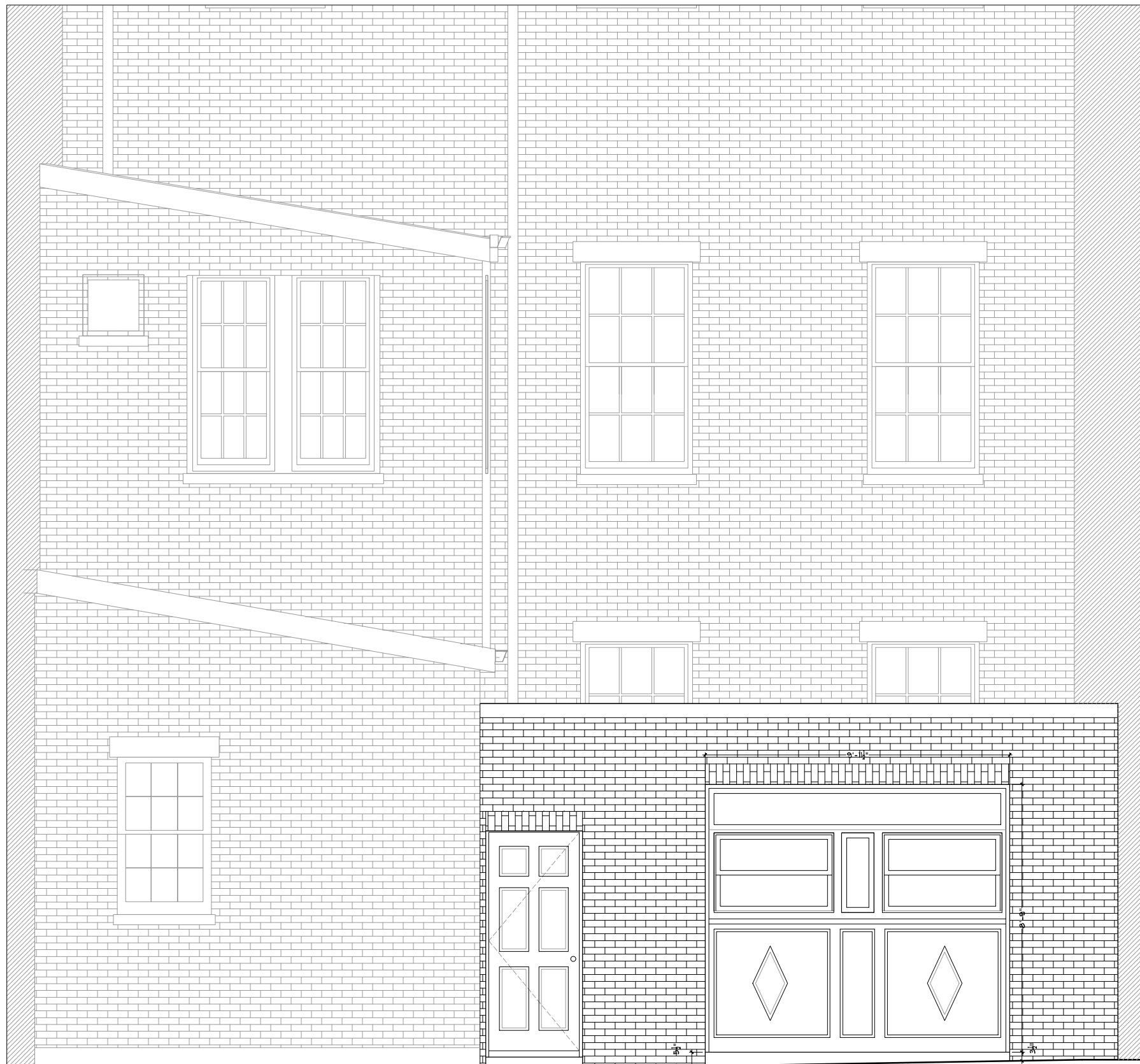
① 28 PINCKNEY STREET - EXISTING ELEVATION FULL: 1/2" = 1'-0", HALF: 1/4" = 1'-0"
