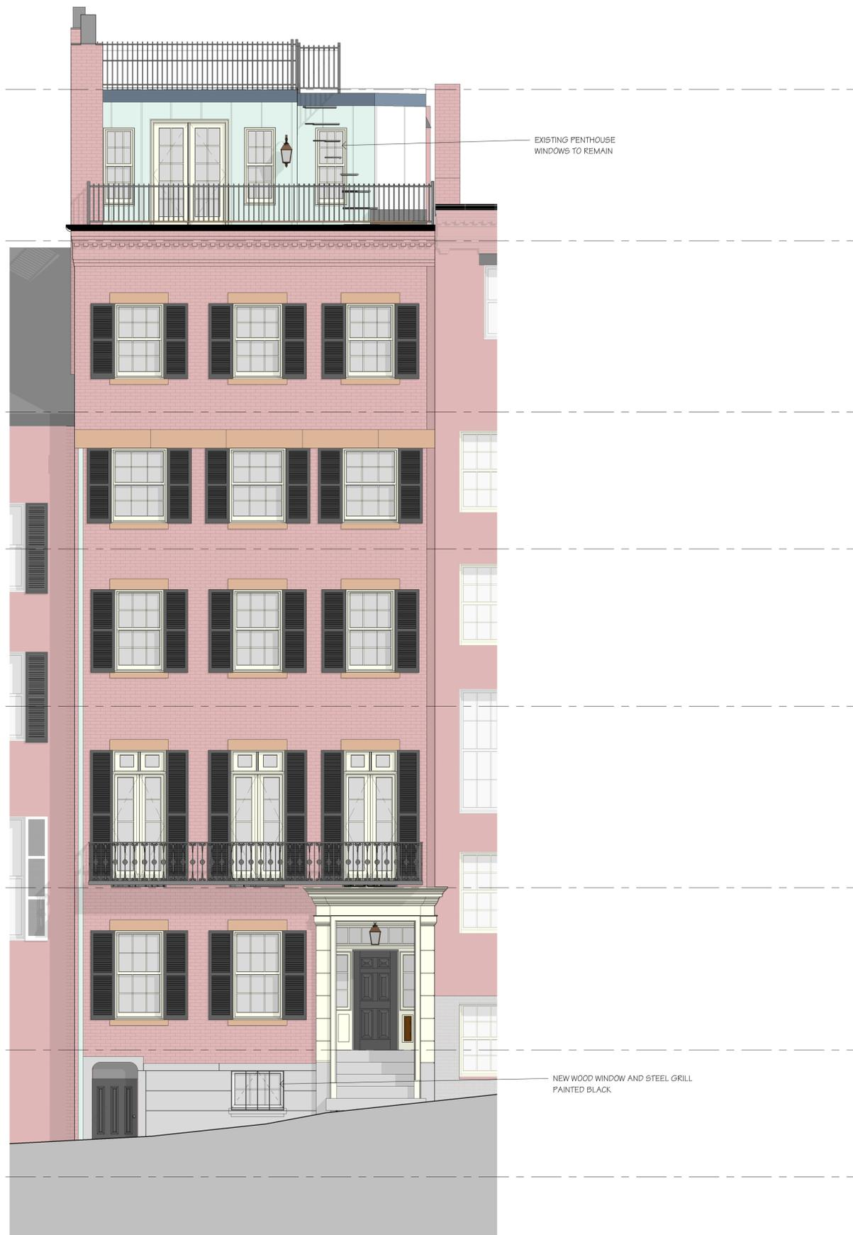
NEW COPPER COPING TO MATCH EXISTING AND TO ALIGN WITH ADJACENT EXISTING PENTHOUSE ROOF
