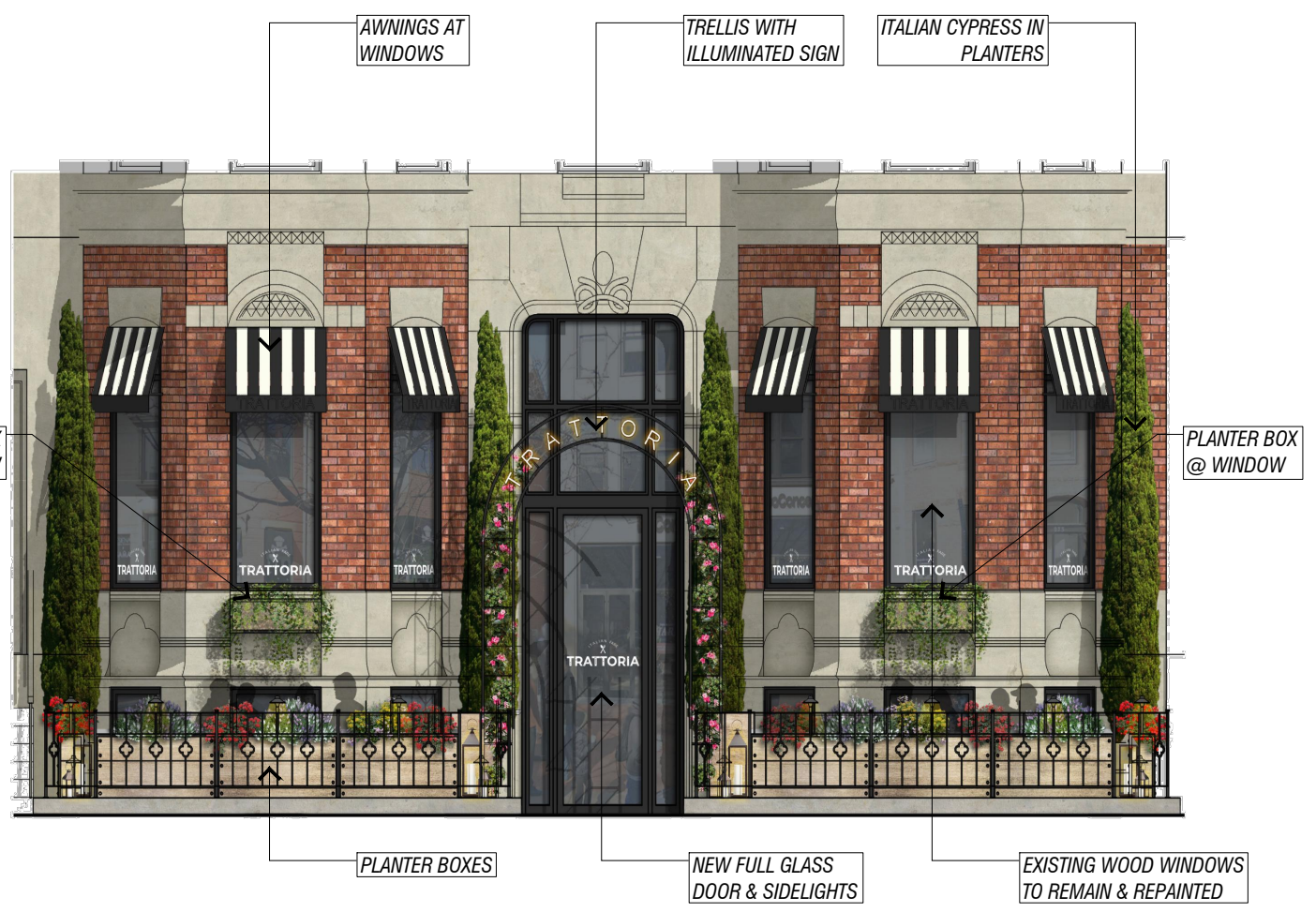
RENDERED ELEVATION - FRONT EXTERIOR PATIO
