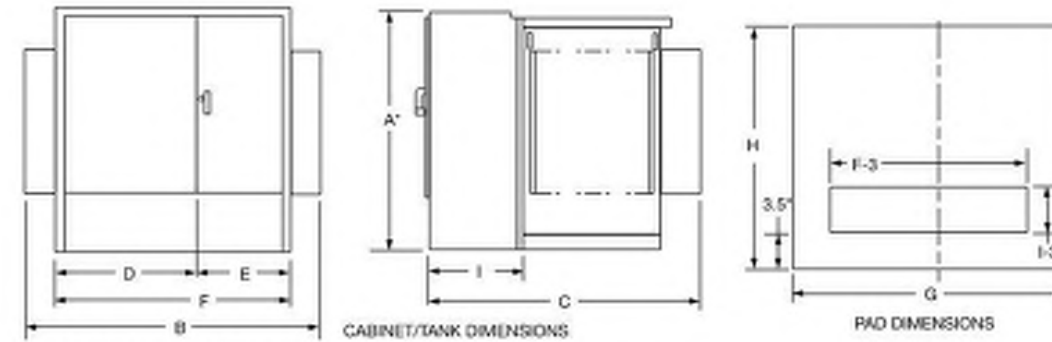
Figure 2. Transformer and pad dimensions.
