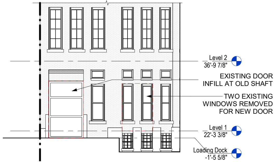
ELEVATION - EXISTING DOCK
