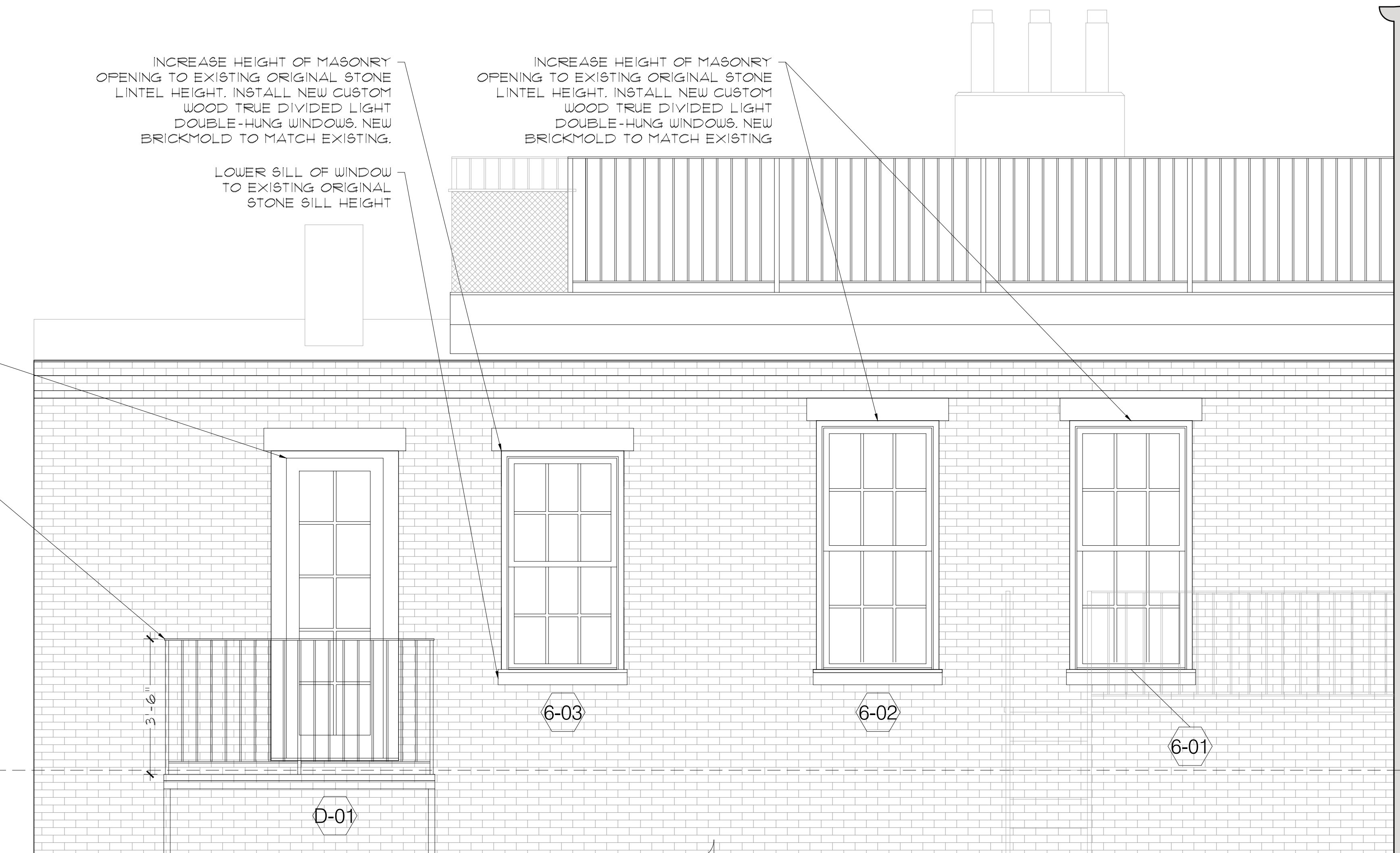
UNIT 6 - PROPOSED EXT. WEST ELEVATION FULL: 1/2" = 1'-0", HALF: 1/4" = 1'-0"
