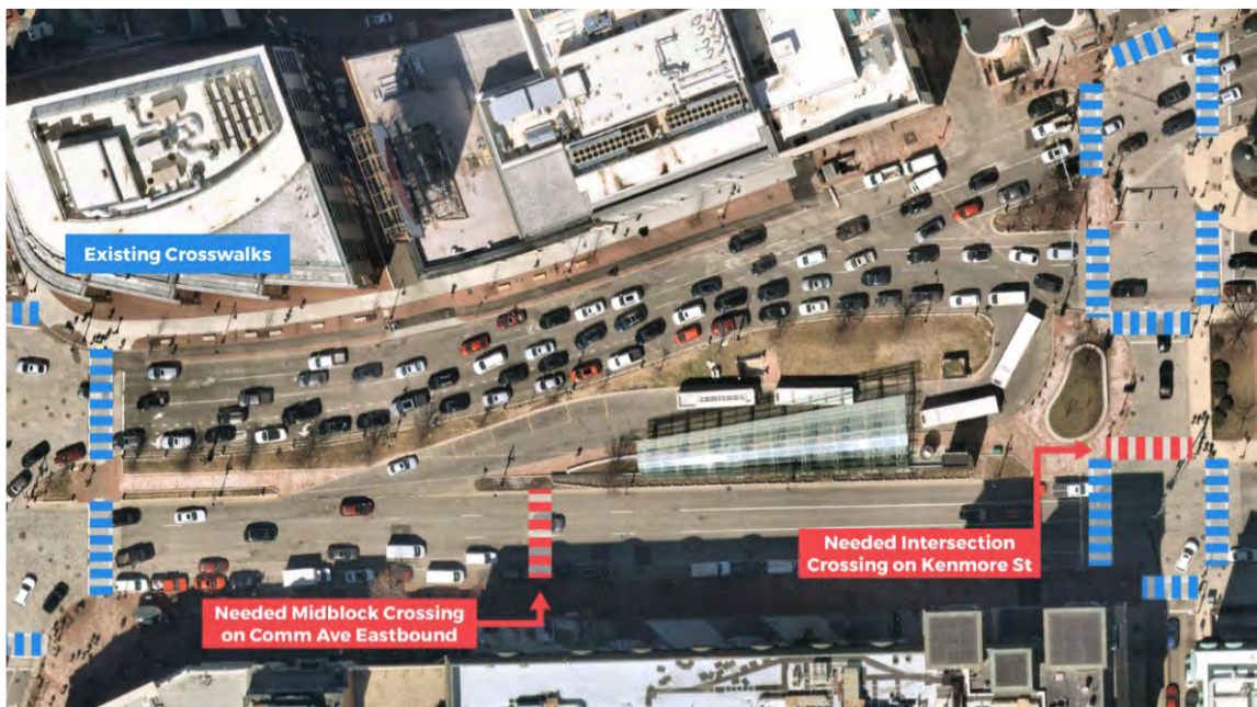
Kenmore Station busway diagram showing needed pedestrian crossings. Image source: Nearmap, March 30, 2023.
