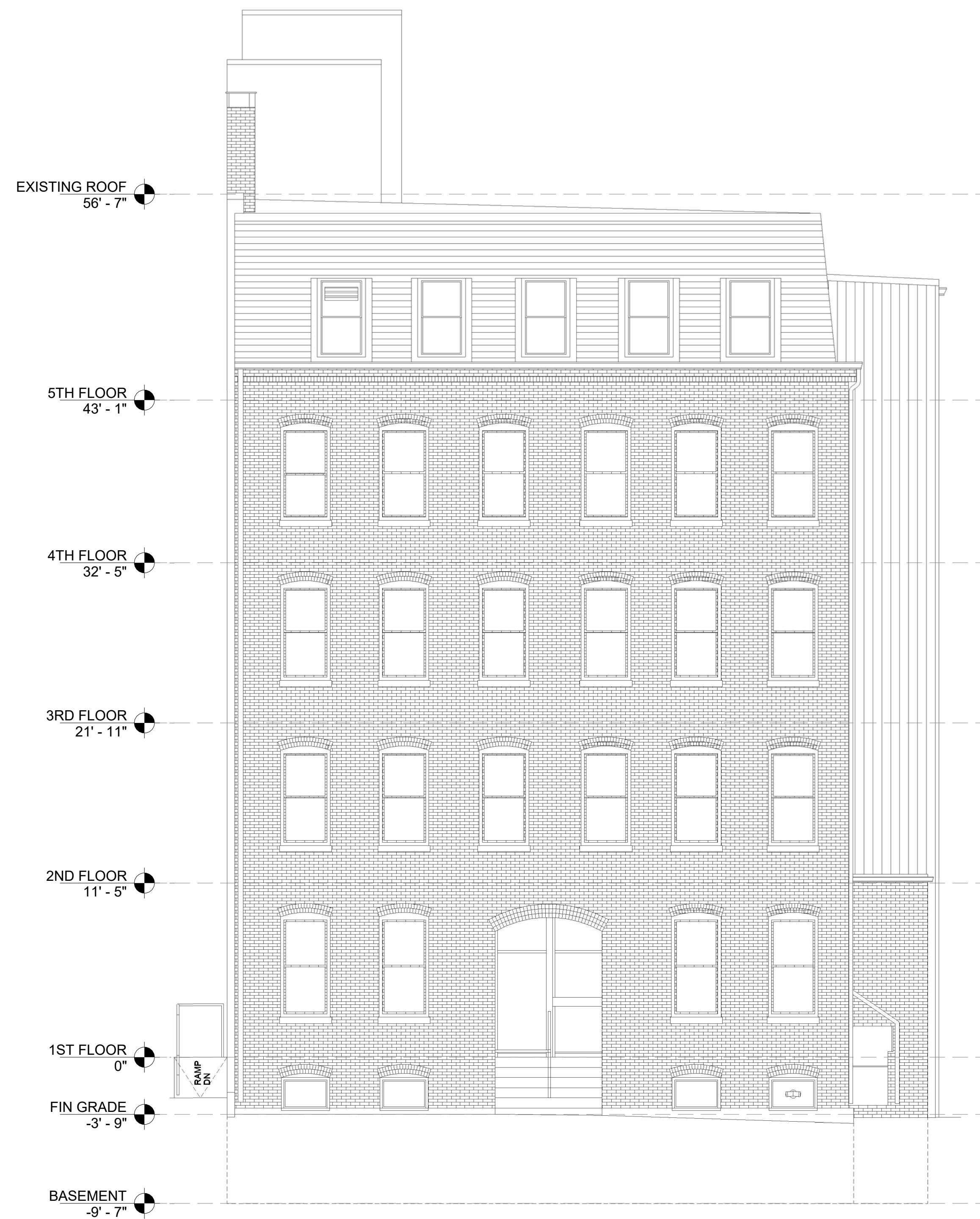
① EXISTING FRONT ELEVATION 3/16" = 1'-0"
