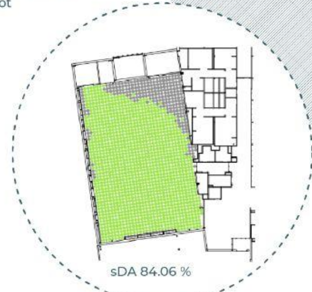
Simulation compared glazing options for optimized daylight performance
