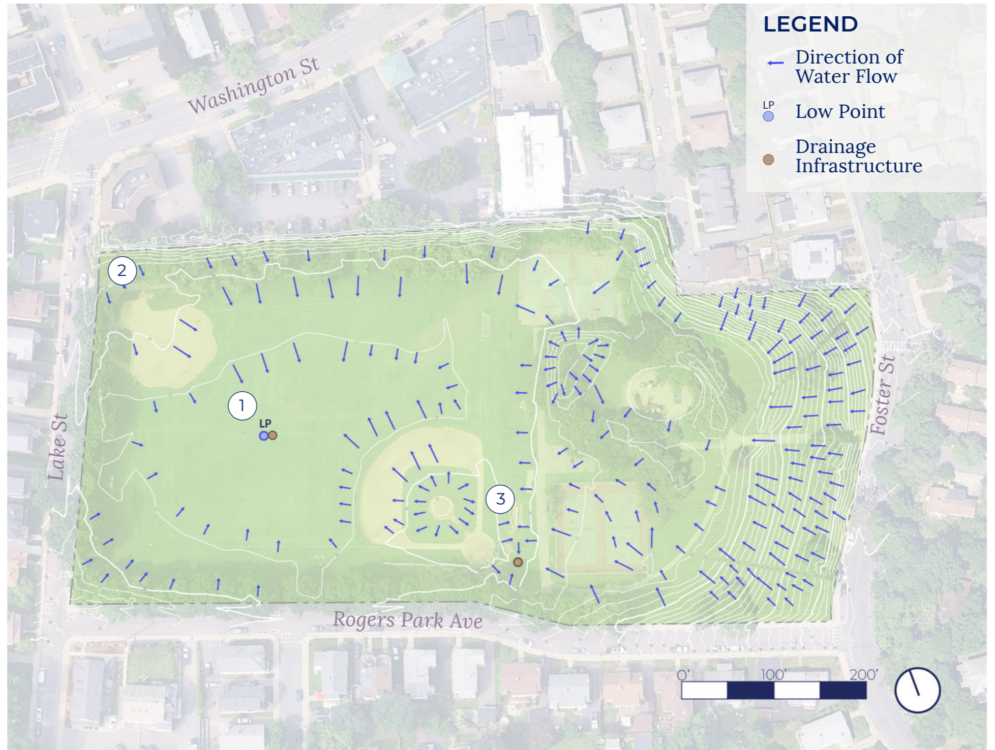
1 Grades pitch toward center of field, causes ponding
