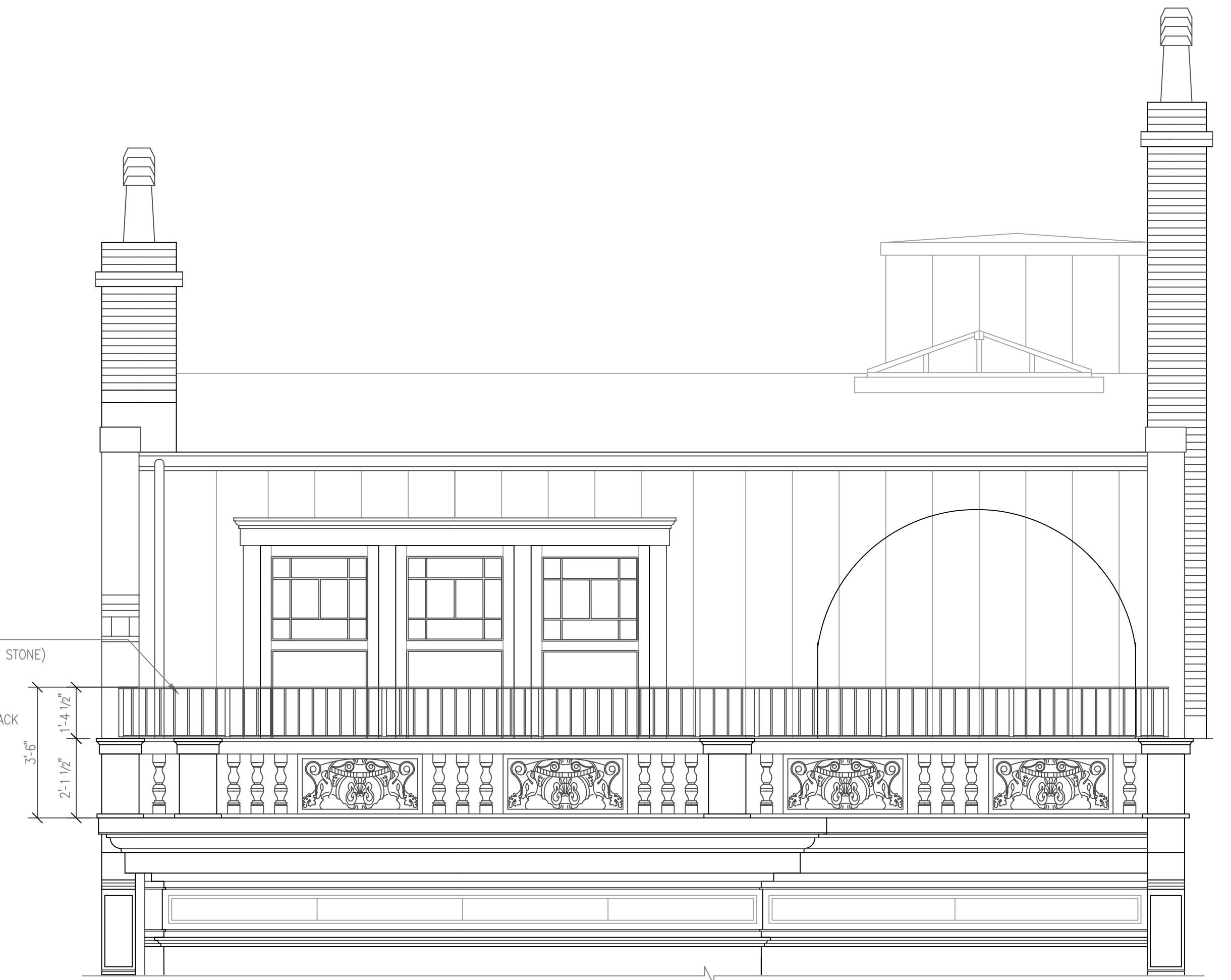
4 PROPOSED TERRACE RAILING ELEVATION (FROM STREET) SCALE: 3/8" = 1'-0"
