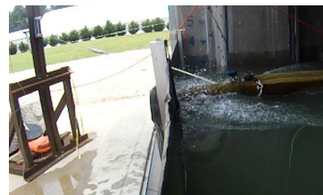
LOG IMPACT TESTING PERFORMED AT ILC DOVER TEST FACILITY
